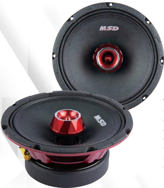
Coaxial Full Range Loudspeaker With Super Bullet Tweeter Woofer: Steel Basket Paper Cone With Cloth Edge 1.5" Voice Coil Tweeter: Aluminium Diaphragm 1" Voice Coil NdFeb Magnet
