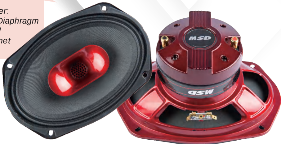
Coaxial Full Range Loudspeaker With Super Bullet Tweeter Woofer: Steel Basket Paper Cone With Cloth Edge 1.5" Voice Coil Tweeter: Aluminium Diaphragm 1" Voice Coil NdFeb Magnet
