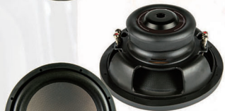
Stamped steel basket subwoofer Pressed paper cone with acrylic dustcap. Foam surround
