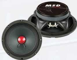
Shallow die-casting aluminium basket mid-woofer Paper cone with cloth surround
