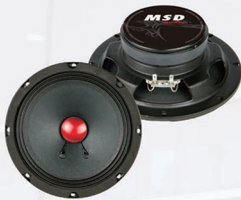
Shallow stamped steel basket mid-woofer Paper cone with cloth surround
