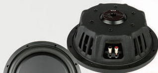
Shallow style stamped steel basket subwoofer PP cone with foam surround
